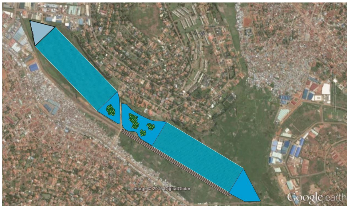
Figure 9- 34: Proposed configuration of the proposed Nakivubo constructed wetland system
