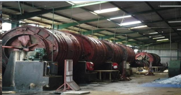
A new set of tanning drums installed during the RECP programme at LIU
