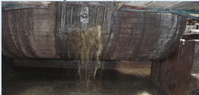
Old leaking drums before RECP at Leather Industries of Uganda (LIU)
